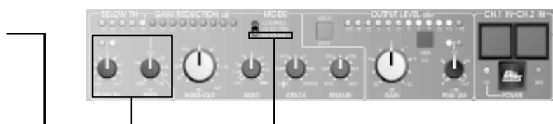
Fig 12.2 HF DE-ESS Controls
