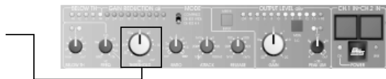
Fig 10.1 Varying the THRESHOLD controls the VCA window on the input signal
